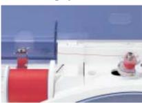
Bobbin winding made easy – wind the thread four or five times around the bobbin, pass it through the guide slot and press the start button. Simple.
