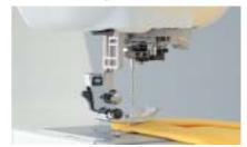
Keeps the presser-foot level for smooth consistent stitching across varying fabric thickness, such as at the start of a seam or when crossing seams.
